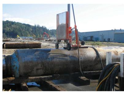
The wire saw was used to cut half way through the steel rolling pin.
